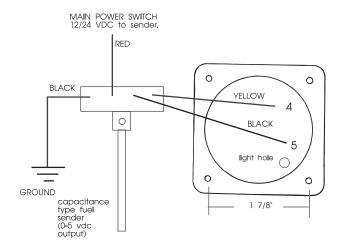
This gauge works with 0-5 volt output senders that have 4 wires.
